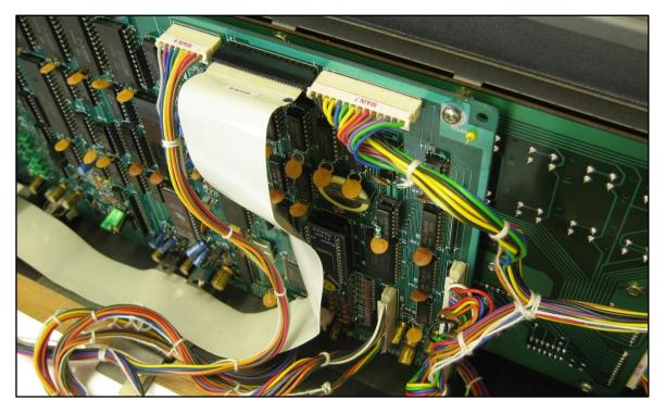
Note the orientation of **CN2** in particular as there are unused pins in the socket on the board.
