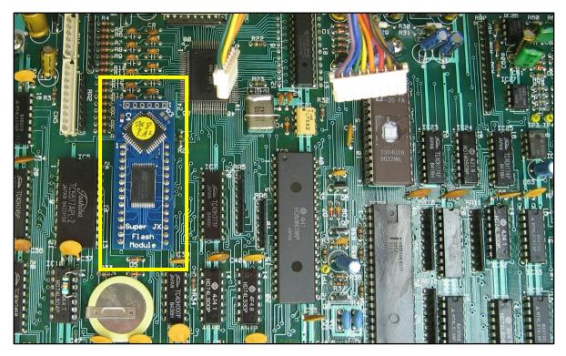
Refit the main board and reconnect all cables. Ensure **CN2** is correct! Close the lid and power up the JX-8P to check correct operation.
