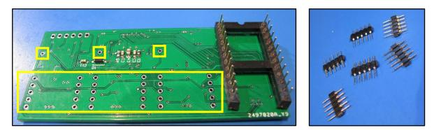
Note that the six pins of **J1** are not connected and do not require header pins.
