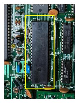
It is recommended that a high quality socket is soldered in place. Such a socket may have been included in the PWM kit if requested.
