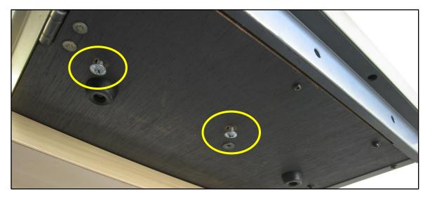
Remove the three screws indicated from both the left and right hand side end cheeks.
