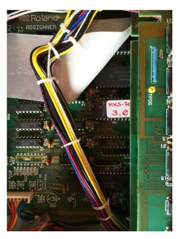
To install newer EPROM A with firmware 3.0, use tool C "IC Integrated Circuit Leg Straightener Tool" to adapt pins to the base.
