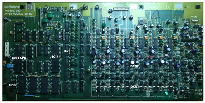
8031 CPU to be replaced with 80C320 CPU IC18 provides the 4051 select signals (X5/X6) IC14 provides the PWM1 and PWM2 select signals
