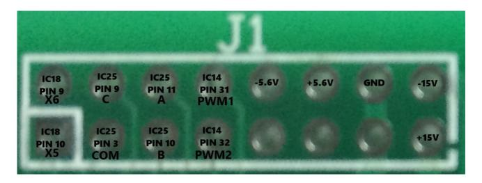
And finally some power..and please note that only one connection is required to each of the +/- 5.6V pins and the GND pin.
