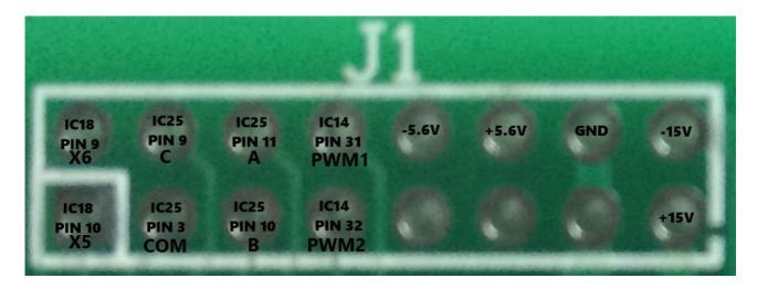
The J1 Header on the PWM board takes in the control signals and power from the soundboard
